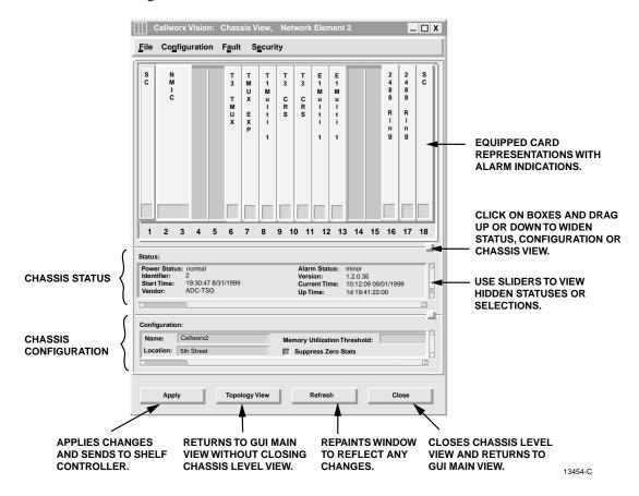
Figure 1-7. Cellworx Shelf Level GUI Screen
